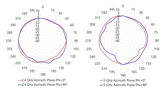
The following figures shows the elevation antenna pattern at 2.4 GHz and 5 GHz radios.
